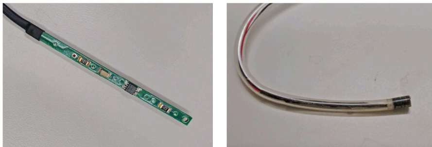
Fig. 2.9 A temperature probe and a shielded temperature probe.
