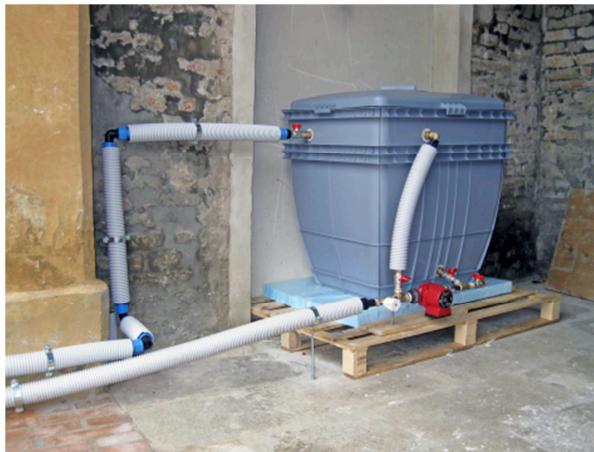
Fig. 2.3 The tank with the pump and micro-meter needle valves.
