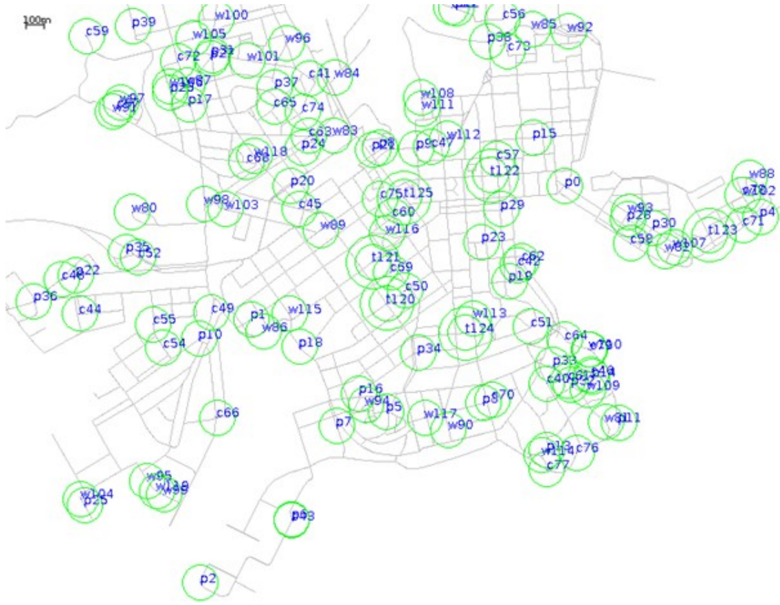
Fig. 25 A screenshot of the networking scenario at the beginning of the simulation with IGeONE; nodes are in blue and their transmission range in green
