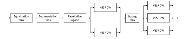
Figure 3. Diagram of the treatment train proposed for the zootechnical farm wastewater.
