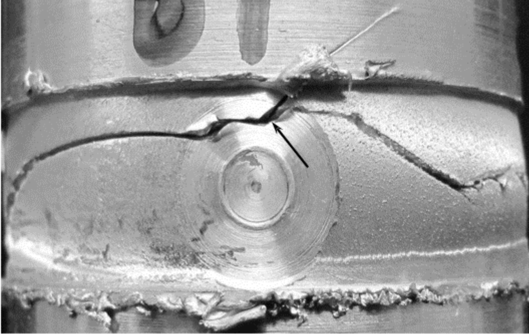
Figura 9-60: Crack initiation site (marked with arrow) in specimen T4 tested in torsion at R = -1 with a shear stress amplitude of 75 MPa.
