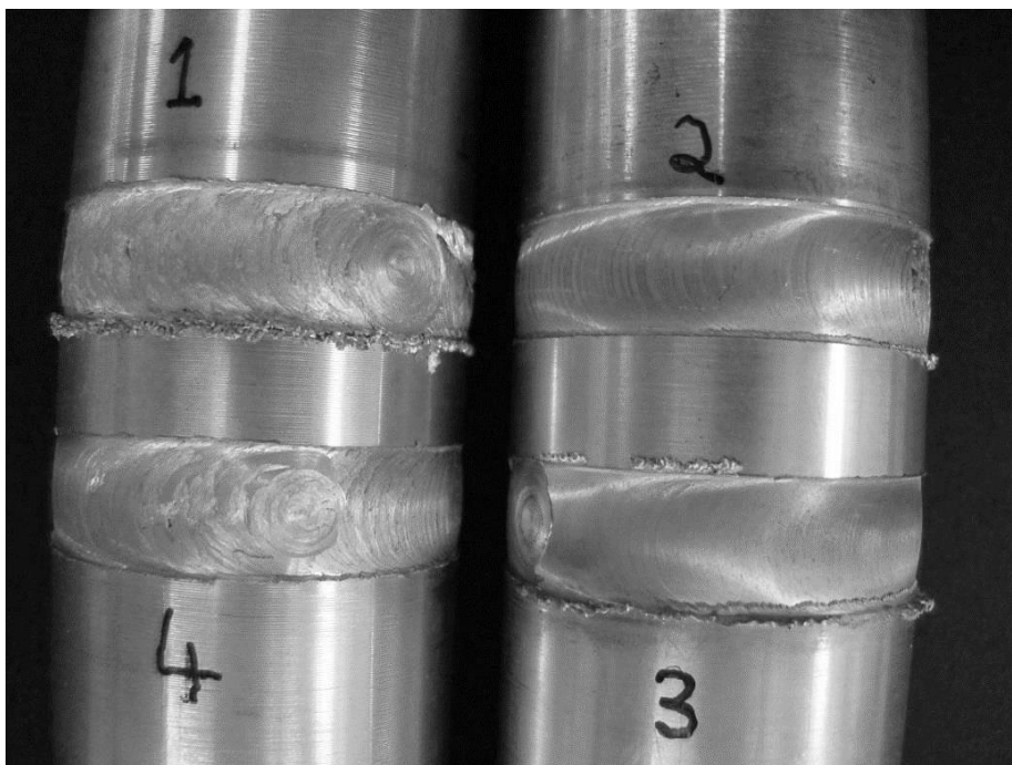
Figura 9-56: Influence of the weld process parameters of plunge depth, rotational feed rate and tool rotational speed on the quality of weld surface finish.
