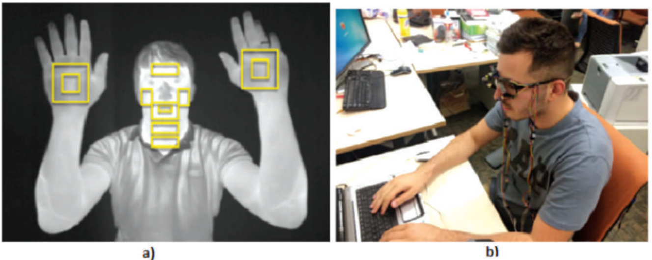
Figure 4. (a) Thermographic data collection points [39], (b) the infrared sensing system installed on an eyeglass frame [40].
