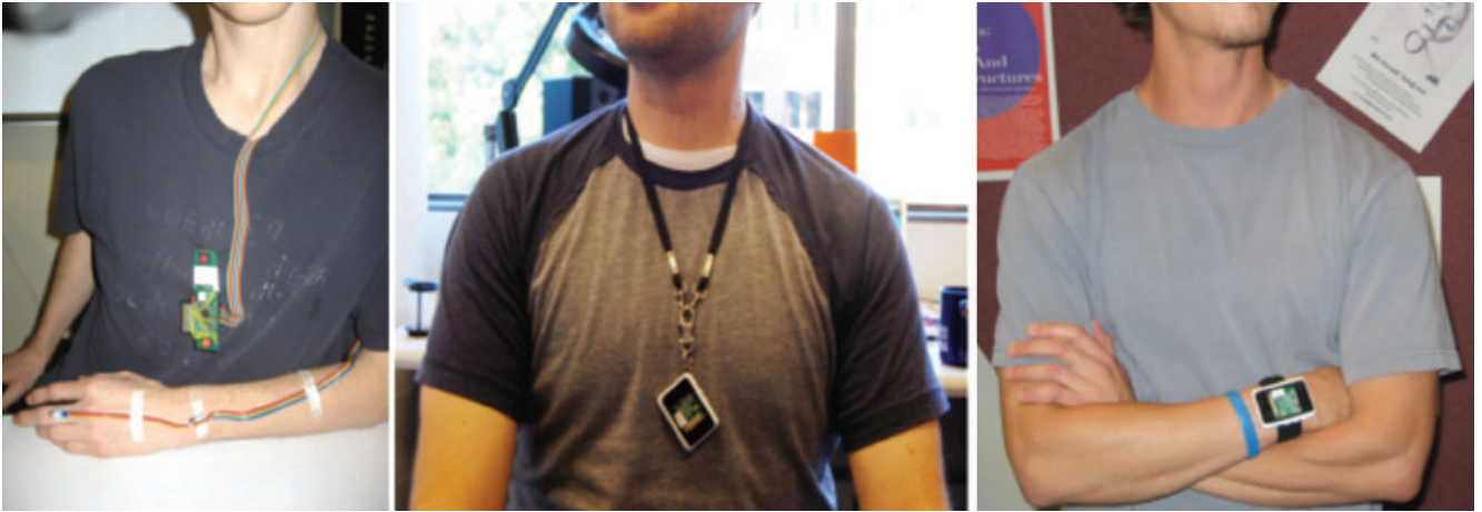
Figure 3. Wearable sensors used for personalized thermal comfort [38]
