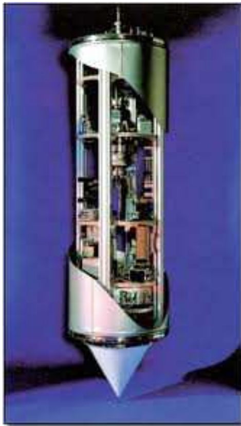
Figure 2.3: The pressurized capsule of the Bremen drop tower
