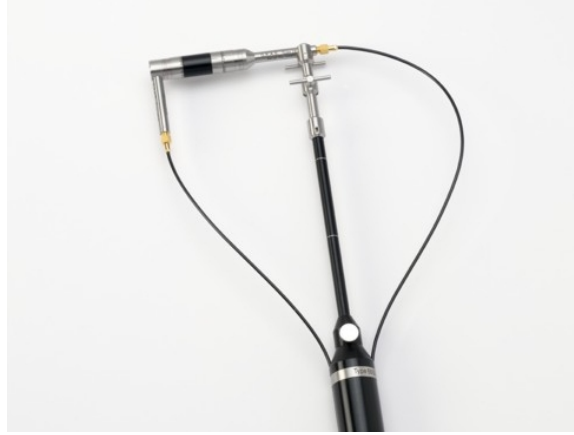
Figure 3.1.3: Example of axial p-p intensity probe: microphones are in face-to face configuration
