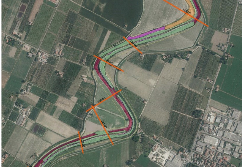
Figure 50. Adorni et al. (2014). Classification of riparian vegetation: detail of final shapefile with polygons of homogeneous features overlapped to a satellite image. Transversal lines are surveyed river cross sections.
