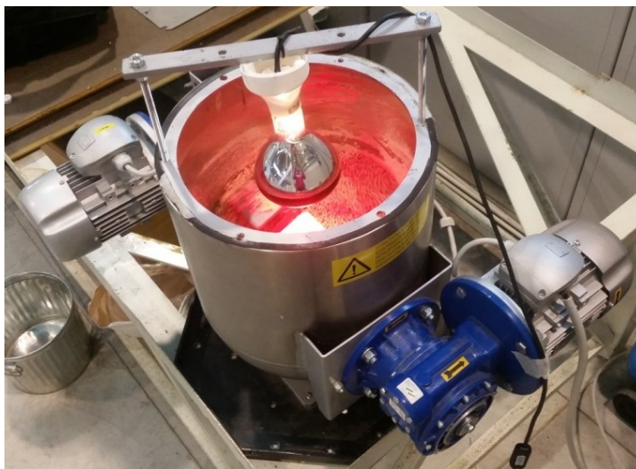
Fig. 6.13 - Infrared drying system
