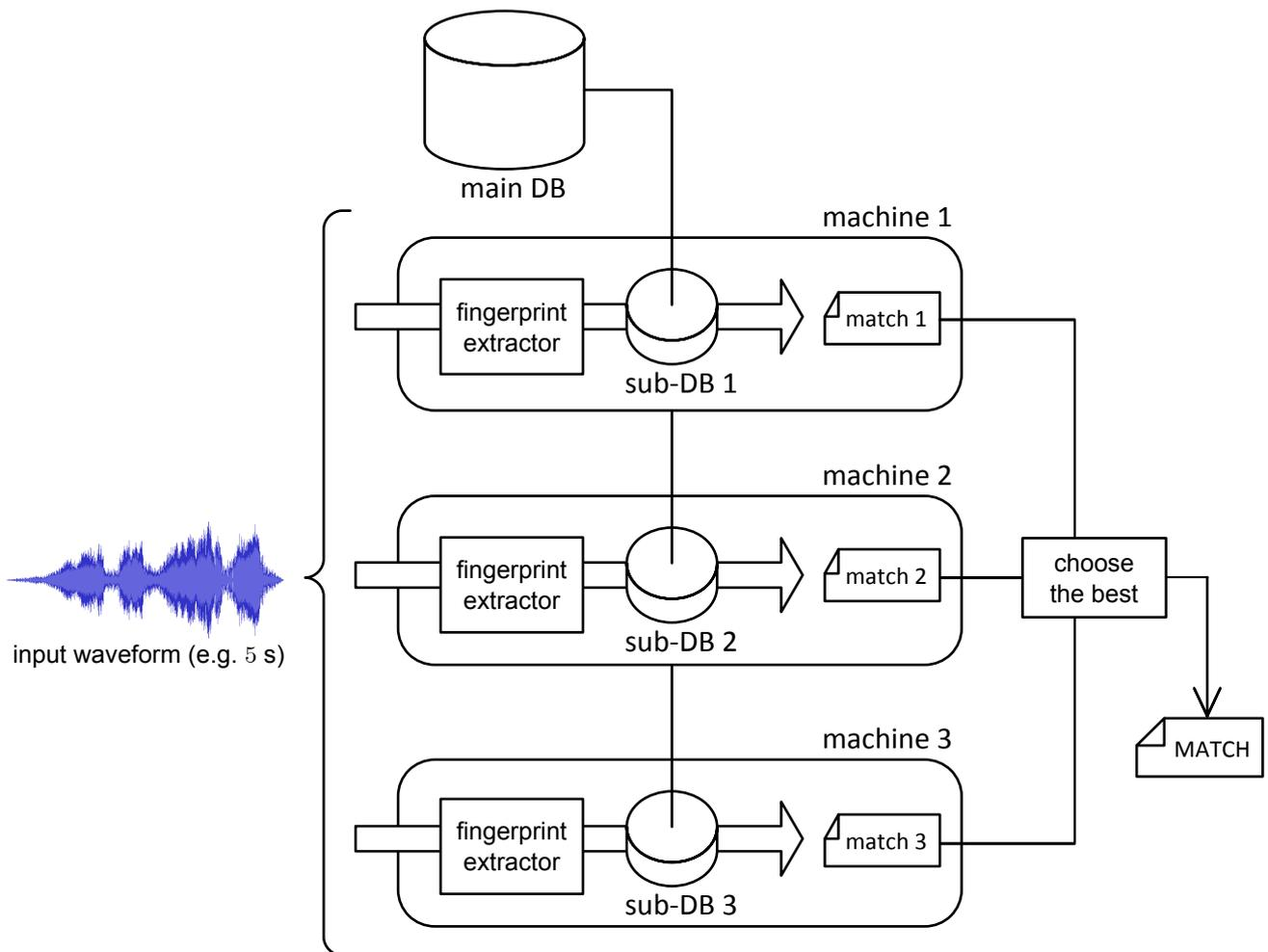
Figure 4.1: Overview of the off-line recognition process, as per the strategy described in section 4.1, in order to overcome memory limitations. For clarity, only 3 sub-databases are depicted here.
