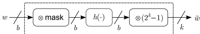
Figure 3.2: Scheme of the algorithm that transforms each single feature vectors from  $b$  into  $k \leq b$  bits. The transformed vectors then populate the hash table used for efficient pattern look-ups.
