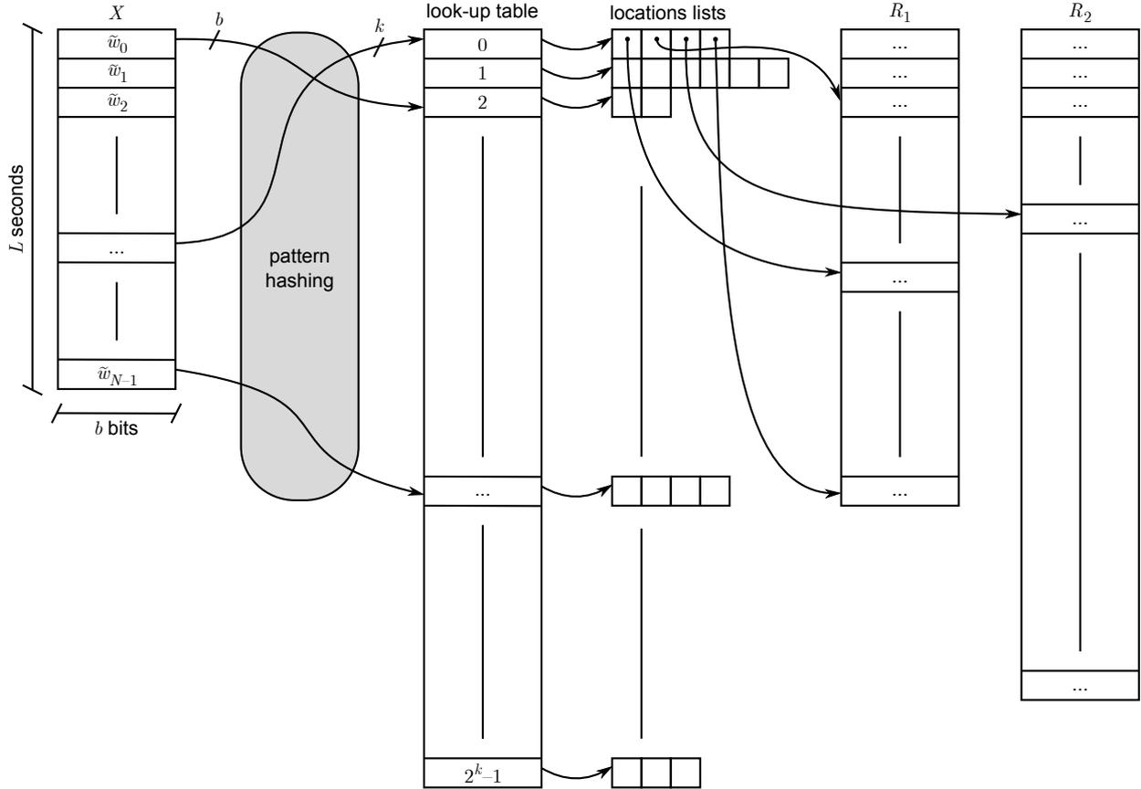
Figure 3.1: The indexing algorithm for fast retrieval of promising alignments between the unknown excerpt and the reference database. The gray block corresponds to the hashing algorithm of Fig. 3.2.
