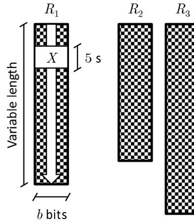
Figure 2.4: The exhaustive search, where  $X$  is the short, unknown audio chunk, while  $R_i$  are the fingerprints of the reference songs stored in the database.
