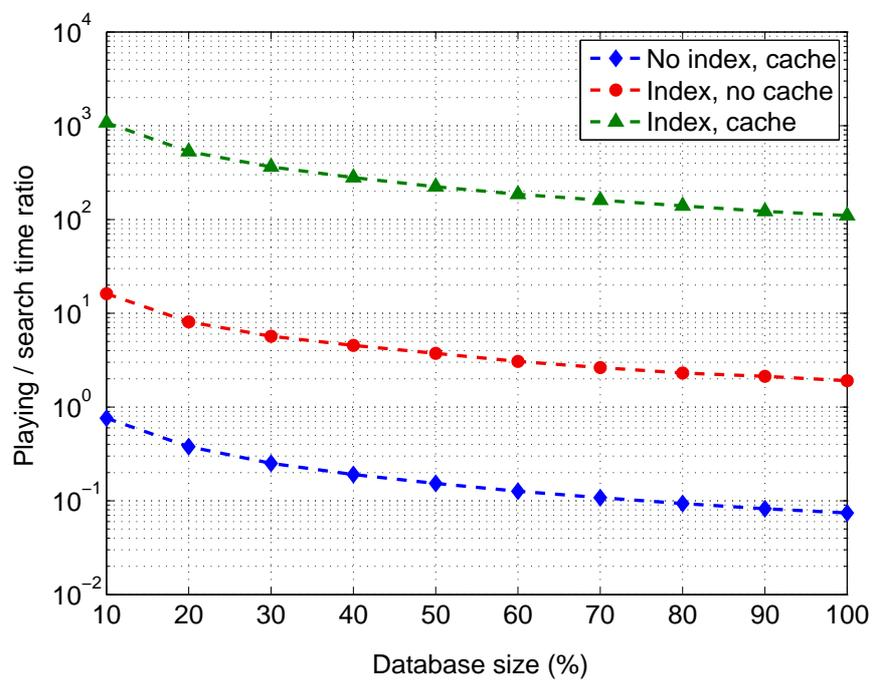
Figure 7.5: Ratio between search time and playing time of the excerpt, as a function of the database size and comparing exhaustive search (which has database on memory), indexing and fully-cached indexing. The index parameter  $k$  is 24.
