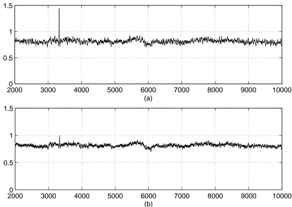
Figure 2.5: Cross-correlations between an unknown excerpt and the matching reference fingerprint. In case (a) the excerpt is undistorted and the synchronization point is easily detectable in correspondence of the high peak. On the other hand, in (b) the test excerpt is corrupted by white noise (SNR of 5 dB), which impairs the peak detection.
