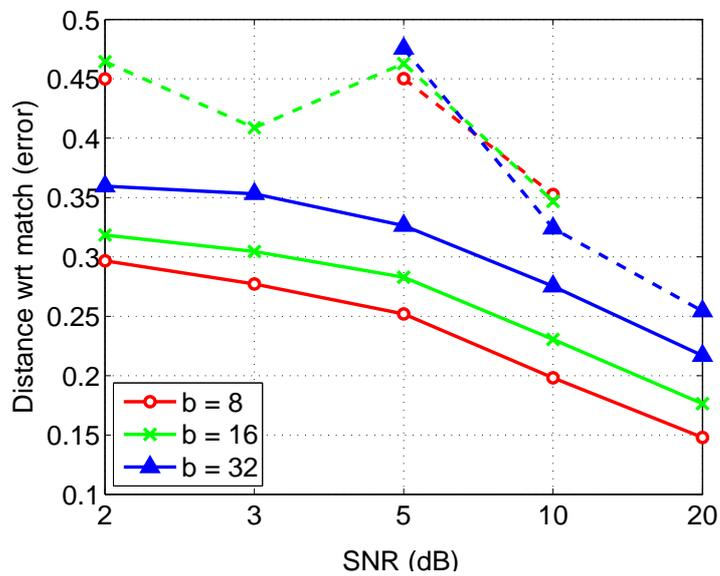
Figure 6.2: In the continuous lines, we depict the distance with respect to match for three different choices of  $b$ . Their respective counterpart in case of error, when errors occur, is represented by the dashed lines.
