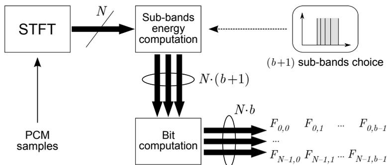
Figure 2.2: The Streaming Audio Fingerprinting (SAF) algorithm.
