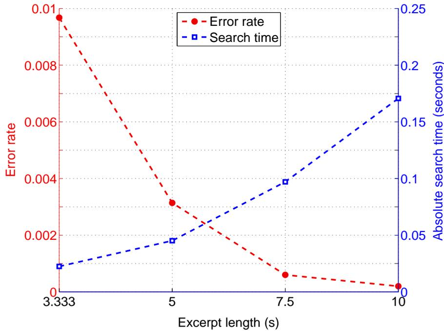
Figure 4.2: Impact of the excerpt length on the error rate and on the search time ( $k = 24$ ).
