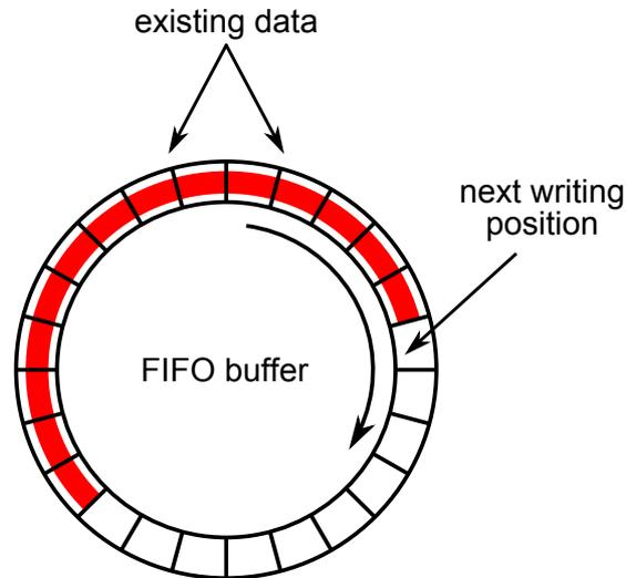
Figure 3.4: The ring buffer used for evaluating the impact of caching the fingerprint database in the computer memory.
