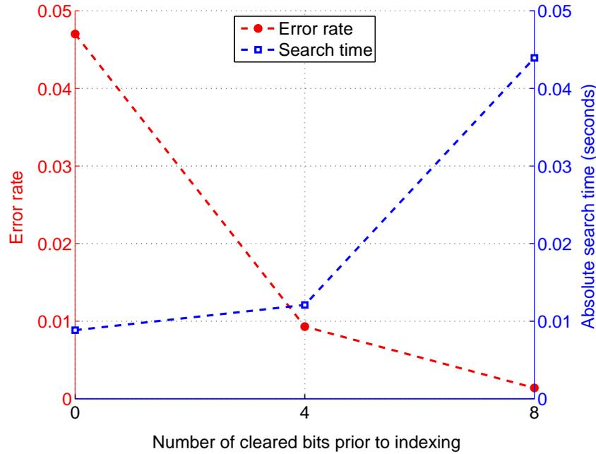
Figure 3.3: Impact of clearing bits in the computed patterns.
