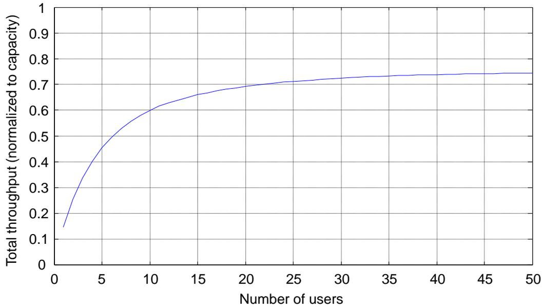
Figure 8.5: Cell throughput in condition of saturation and in the hypothesis of no users leaving the system.
