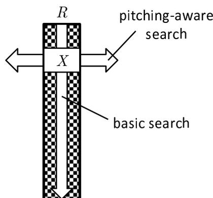
Figure 5.3: The proposed search for combating pitching, where  $X$  is the short, unknown audio chunk, while  $R$  is the fingerprint of a reference song.
