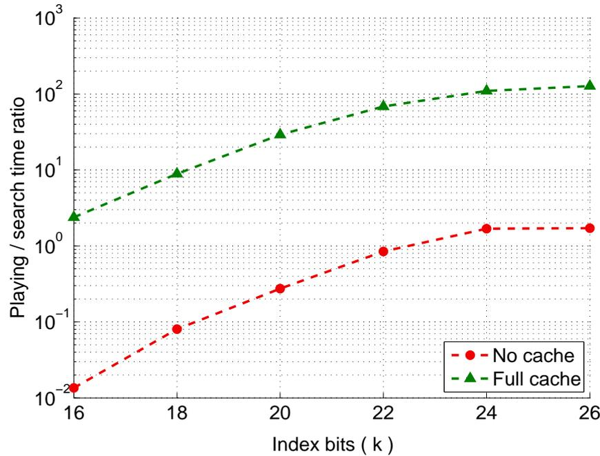
Figure 7.2: Ratio between search time and playing time of the excerpt, as a function of the index parameter  $k$ .
