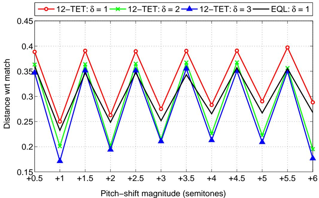
Figure 5.7: Given  $b = 32$ , normalized Hamming distance against the correct match as a function of both the pitch-shift magnitude and  $\delta$ .
