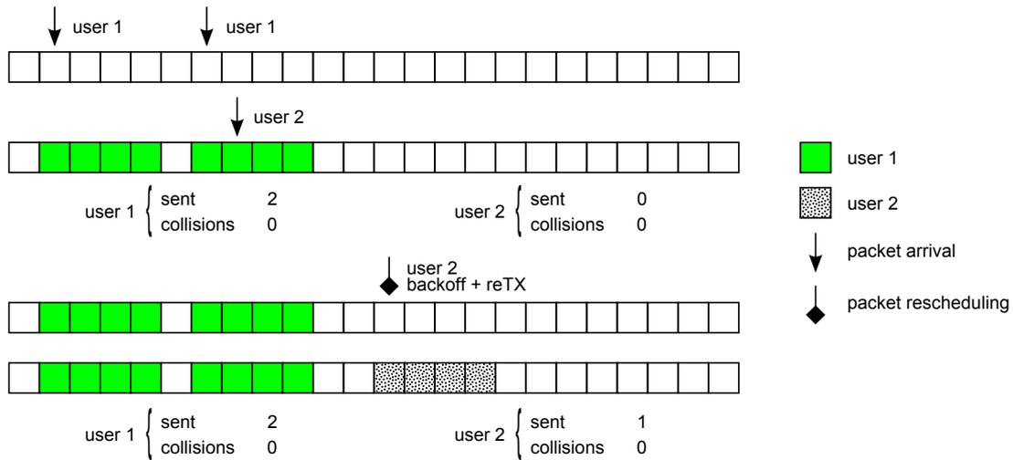
Figure 8.1: An example of backoff rescheduling when the current user senses a busy channel. For clarity, a packet is here only 4 slots long, instead of 64.
