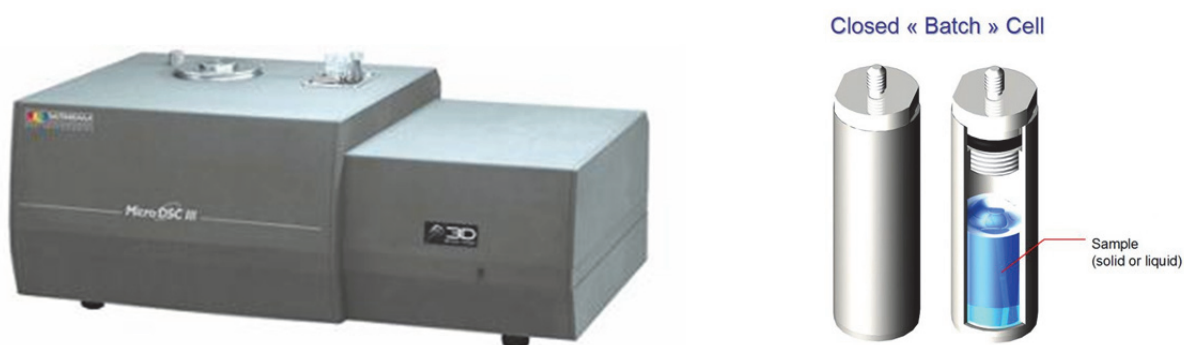
Figure 18. Micro-DSC Setaram III and closed “batch” cells.
