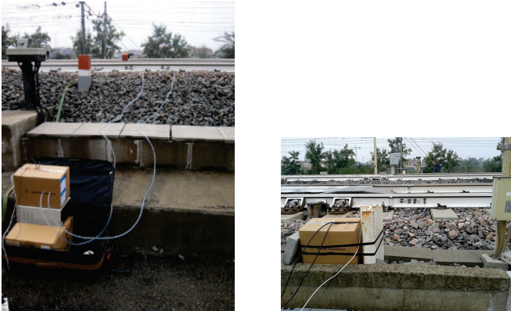
Fig. 5.22 Experimental set ups: on the left the first disposition, with long plastic tubes, and the stethoscopes placed on the odd railway; on the right the reduced tubes.
