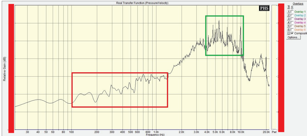
Fig. 5.32 Impedance of the 1200 rpm washing machine with motor damaged. The data are confidential, so the vertical scale has been omitted.
