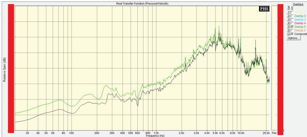
Fig. 5.35 Impedance of the 1400 rpm washing machine with rotor issue (black) and with the 1200 rpm machine working on the background (green). The data are confidential, so the vertical scale has been omitted.
