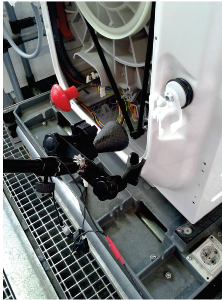
Fig. 5.30 The acoustic horn hosting the Microflow p-v match size probe, placed in the back of the washing machine.
