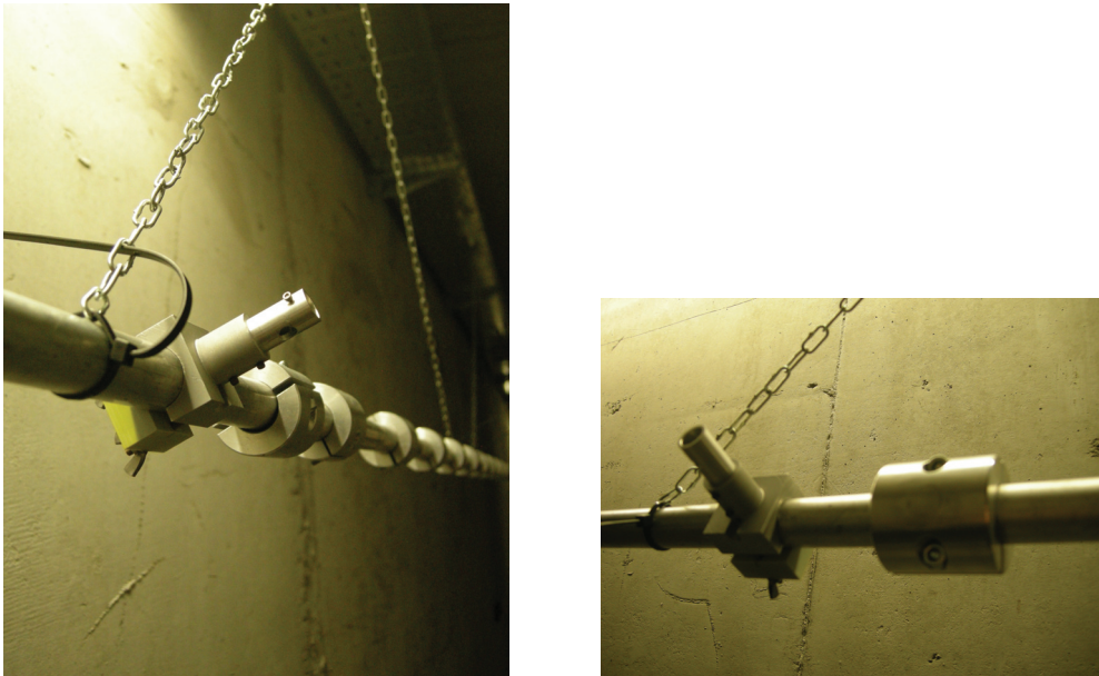
Fig. 4.4 The progressive plane wave tube inside Larix, which has been modified in order to insert the probe at different points through a series of holes: on the right the last hole, 10,8 m far from the source, used for the calibration.
