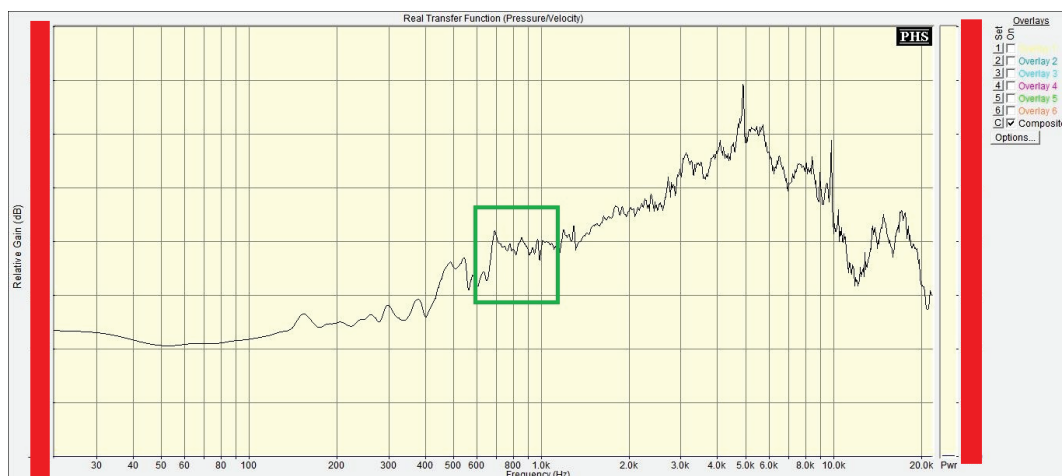
Fig. 5.38 Impedance of the 1600 rpm washing machine with damaged motor and belt. The data are confidential, so the vertical scale has been omitted.
