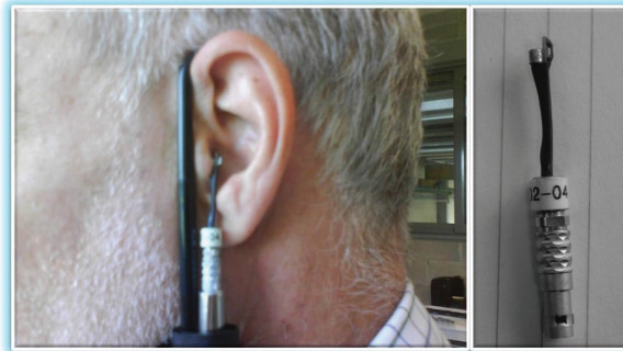
Fig. 5.2 Set up of the first tympanometric test with a p-v commercial microprobe.
