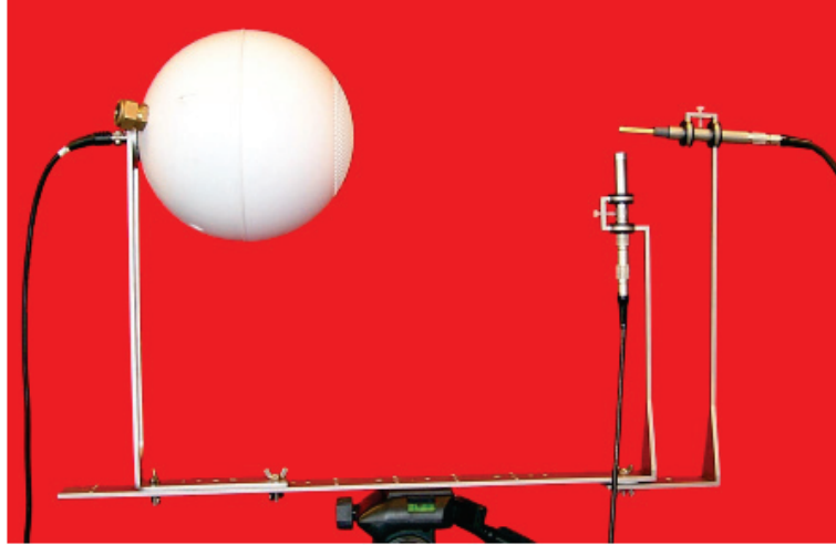
Fig. 2.1 Piston in a sphere set up for the calibration at high frequencies.
