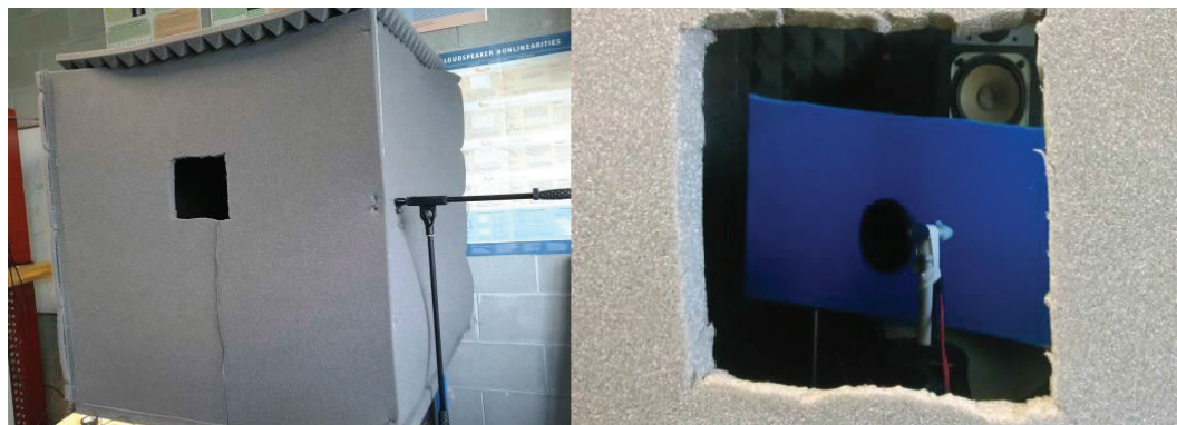
Fig. 3.29 Noise-insulating 1 m 3 chamber .
