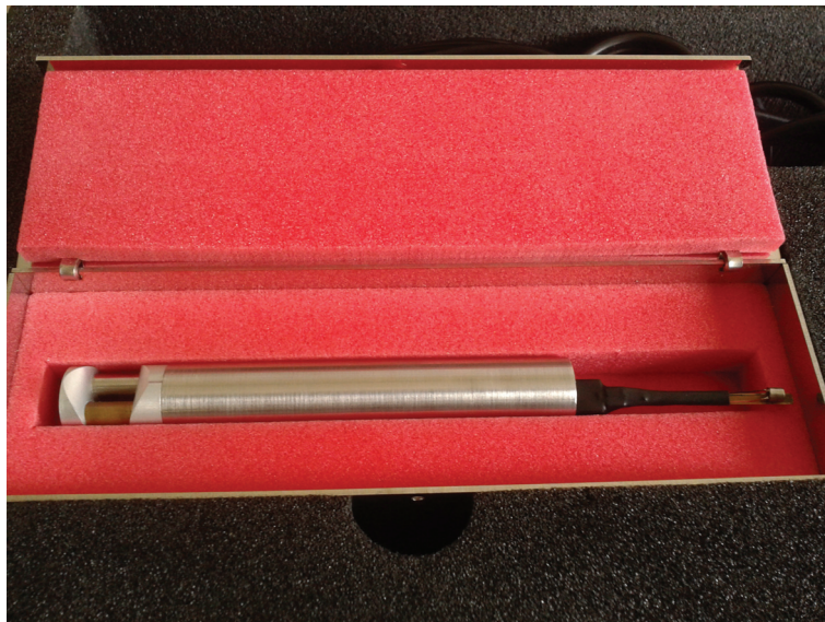
Fig. 2.11 The pressure velocity probe which has been calibrated at Microflow and at Ferrara.
