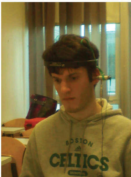
Fig. 5.7 The prototype probe for p-v tympanometry is fitted inside the ear canal at normal pressure conditions.
