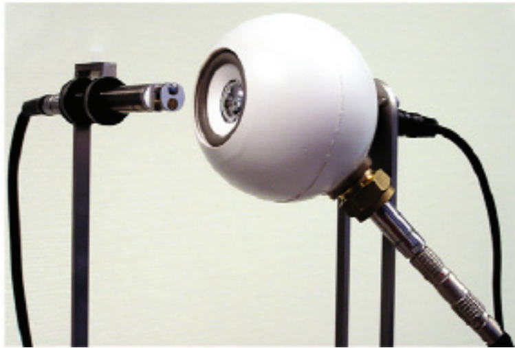
Fig. 2.5 The setup used for the calibration at low frequencies.
