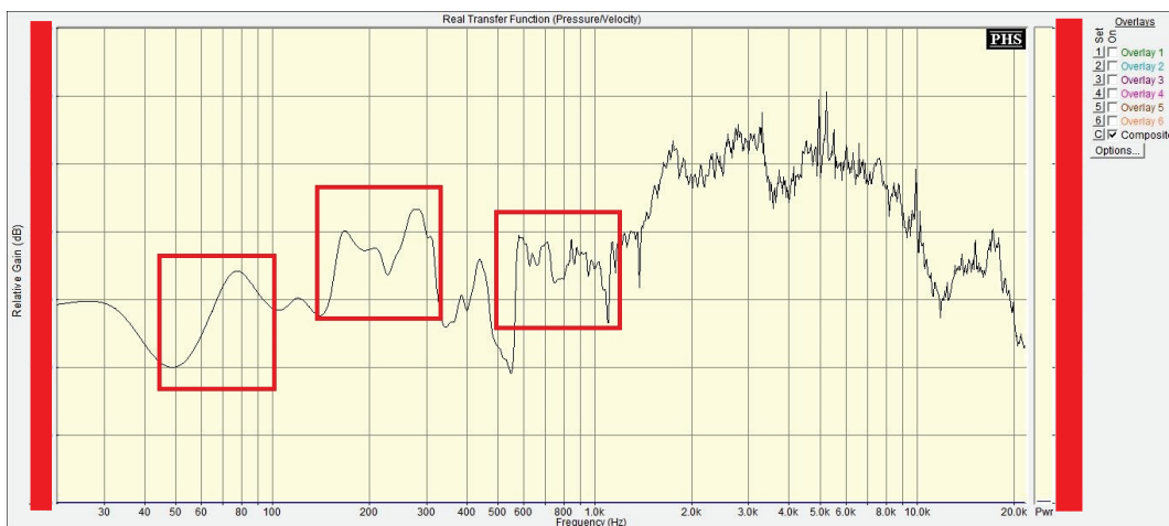
Fig. 5.33 Impedance of the 1200 rpm washing machine with rotor issue. The data are confidential, so the vertical scale has been omitted.
