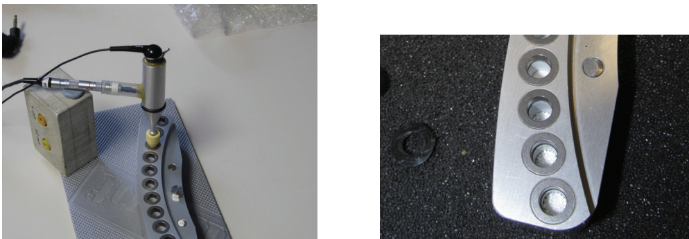
Fig. 5.11 Experimental set up: the tympanometric prototype on the left, a particular of the rack of a capsule filling machine on the right.
