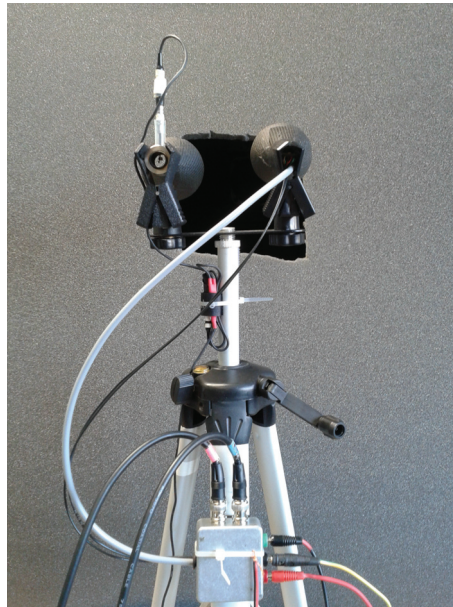
Fig. 4.11 Tripod holding the probes for comparison calibration.
