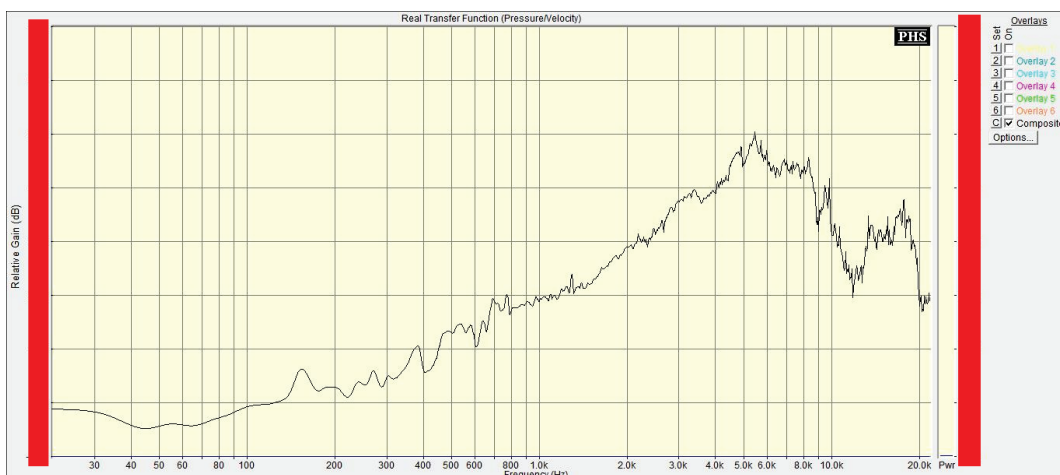
Fig. 5.36 Impedance of the functioning 1600 rpm washing machine. The data are confidential, so the vertical scale has been omitted.
