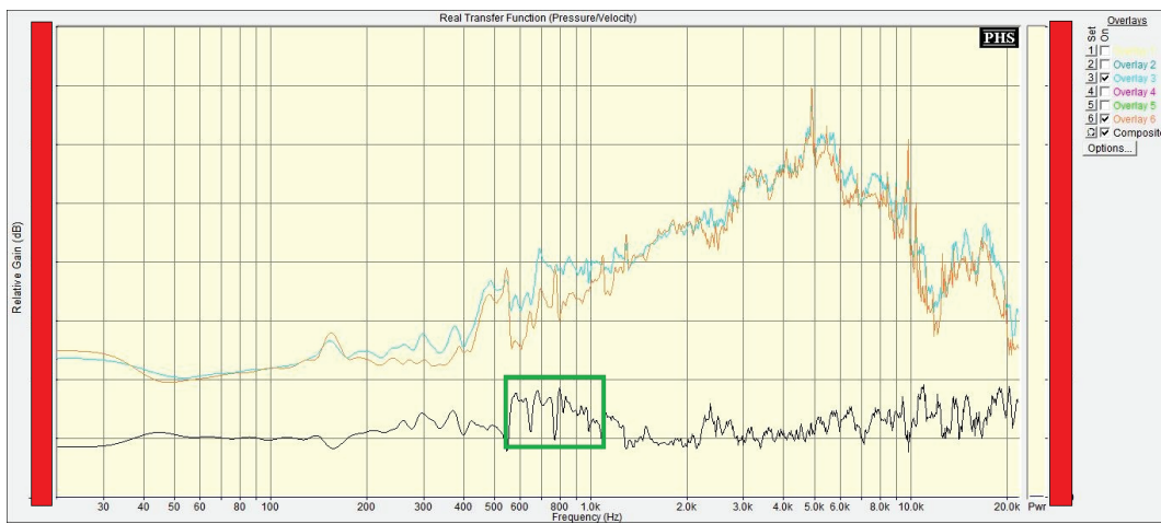
Fig. 5.39 Difference of impedance between the 1600 rpm washing machine with damaged motor and belt and the one with only damaged motor. The data are confidential, so the vertical scale has been omitted.
