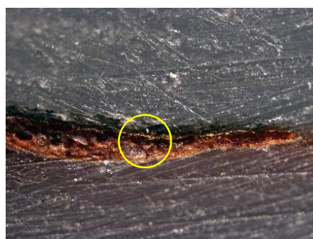
Figure 8.29. Cross section image of the sample B5, presence of gold leaf, magnification 200X
