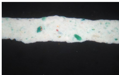
Figure 9.57. Cross section images of the sample SA5, magnification 180X
