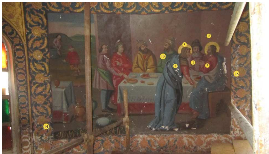
Figure 8.7. Samples B1-B5 and B13-B15 from the first wall painting in the church of Surb Betghehem (Photo by: Y. Hamzavi).
