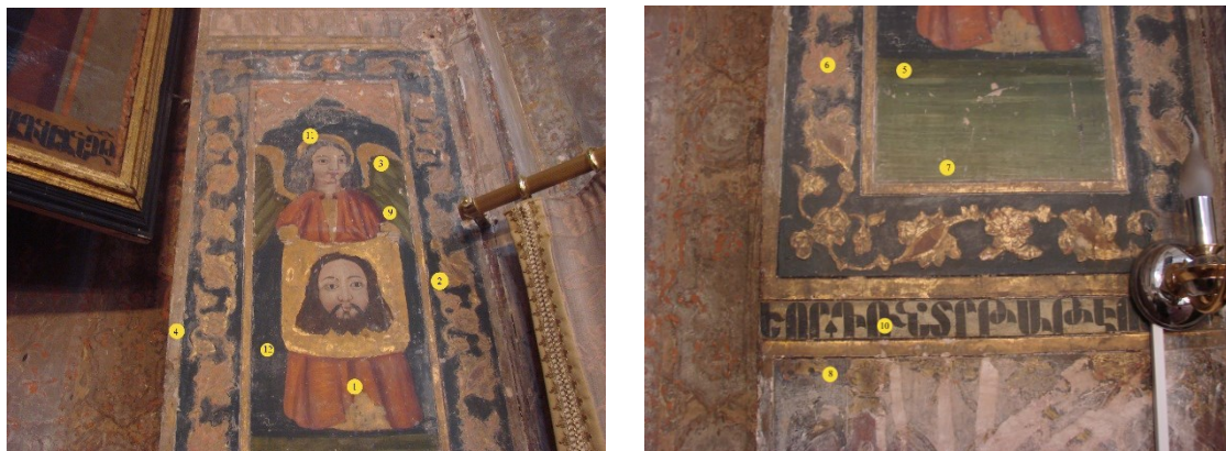
Figures 9.6 & 9.7. Sampling points on the selected wall painting, the church of Surb Stepanos
