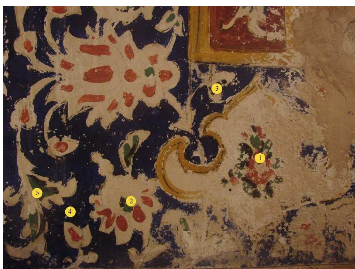
Figure 7.5. Sampling points on the selected wall painting, the church of Surb Astvatzatzin
