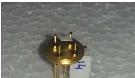
Figure 4.51: Photo of the device made of ECS 14 powder in paste formulation without glass frit and with addition of ethanol.
