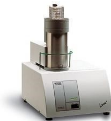
Figure 3.22. Thermogravimetric balance Netzsch STA 409 PC Luxx, located at the Physics and Earth Sciences' Department of the University of Ferrara.
