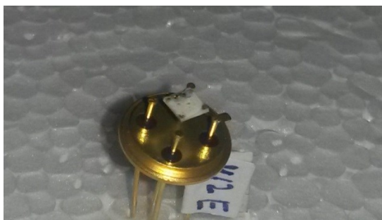
Figure 4.54: Photo of the device made of ECS 12 powder in paste formulation without glass frit and with addition of ethanol.
