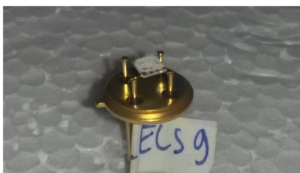
Figure 4.48. Photo of the device made of ECS 9 powder in paste formulation without glass frit.
