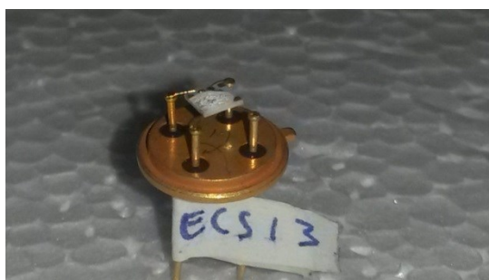
Figure 4.50. Photo of the device made of ECS 13 powder in paste formulation without glass frit.
