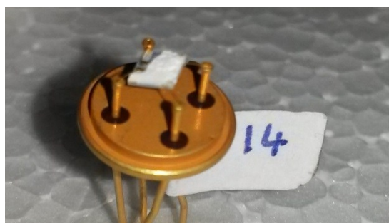
Figure 4.39. Photo of the device made of ECS 14 powder in complete paste formulation with the addition of ethanol.
