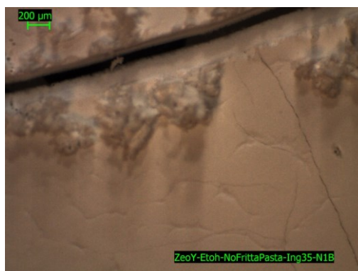
Figure 4.37. Film obtained by using Y(1) zeolite dispersed in organic vehicle and ethanol.
