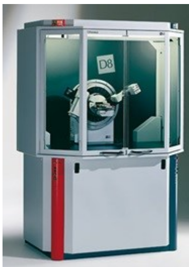
Figure 3.21. XRD Diffractometer Bruker, located at the Physics and Earth Sciences' Department of the University of Ferrara.
