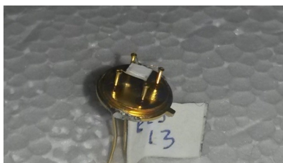
Figure 4.54. Photo of the device made of ECS 13 powder in paste formulation without glass frit and with addition of ethanol.
