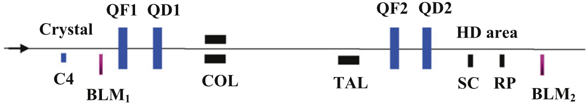
Figure 6.6: The simplified layout of the UA9 experiment. The crystal primary collimator C4 is located upstream the quadrupole QF1. The TAL acting as a secondary collimator-absorber is upstream the quadrupole QF2. Some target, SC or RP, in a high dispersion HD area is used to measure off-momentum particles produced in the collimation process. QD1 and QD2 are the defocusing quadrupoles.
