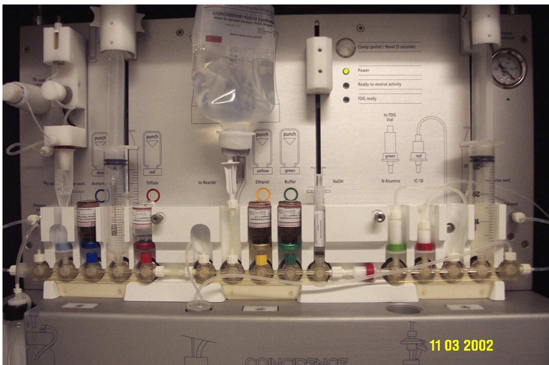
Figure 9: Hardware of an Mx TRACERlab with a disposable ^{18}\text{F} -FDG cassettes and reagents assembled (G.E.m.s)
