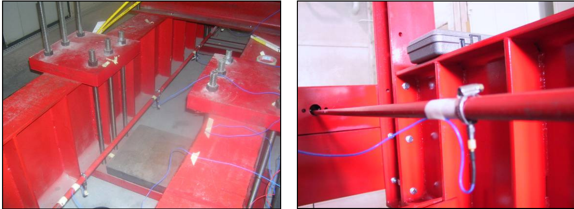
Figure 3.7 – Accelerometers arrangement and fixing system adopted by metallic wrappers
