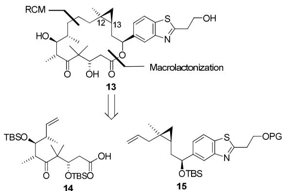
**Scheme X-1** Retrosynthetic analysis of **13**: disconnections into two building blocks.
