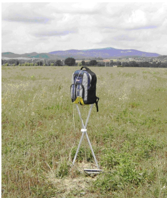
Figure 3.12: example of acquisition of the spectrum with backpack placed on the tripod at 1 m height above the ground.
