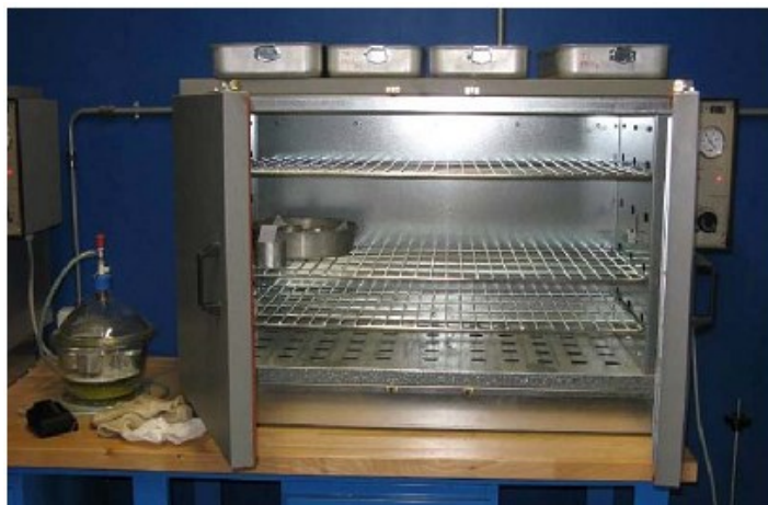
Figure 4.1: ventilated oven used to dry the soil samples.
