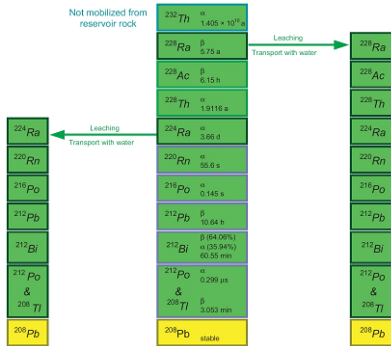
Figure 1.18: decay chain of ^{232}\text{Th} where are highlighted the possible points in which the condition of personal equilibrium is broken.
