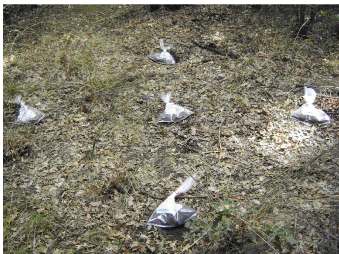
Figure 3.14: example of the soil samples arrangement with respect to the central point in which is realized the measurement of gamma-ray spectroscopy in situ.
