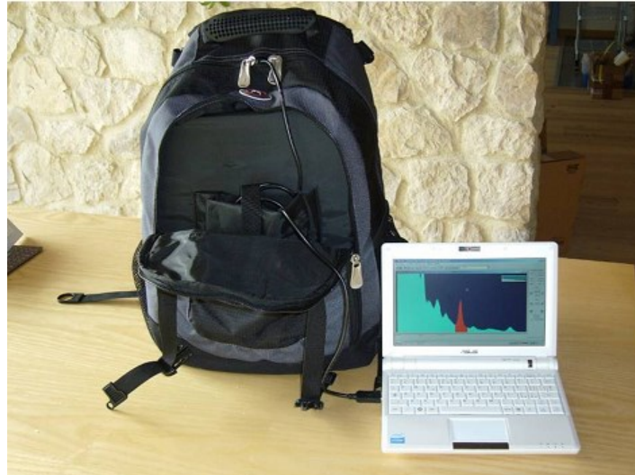
Figure 3.8: the ZaNaI_1.0L system configuration set-up in a backpack.
