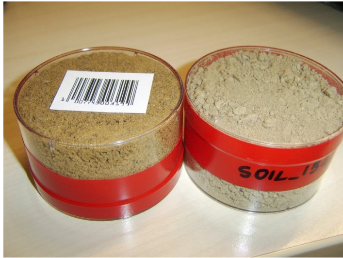
Figure 4.2: soil samples ready to be analyzed with MCA_Rad system.
