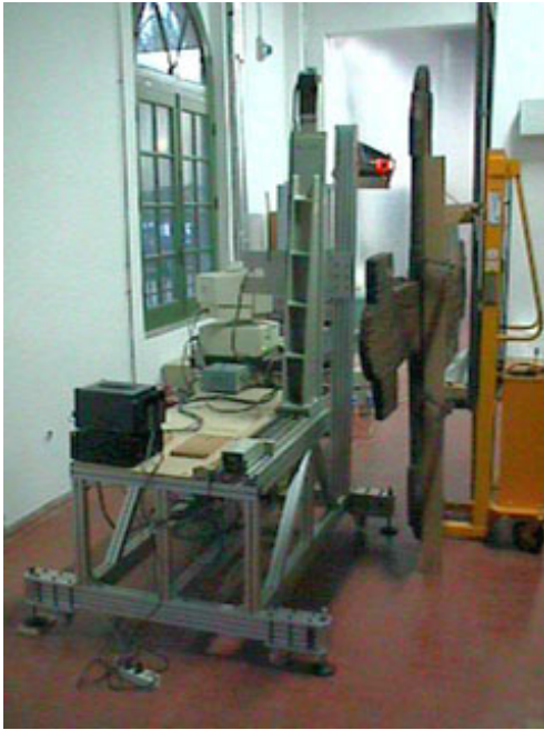
Fig. 2.6. Image and components scheme of reflectographic scanner system of INO, Florence. [14]
