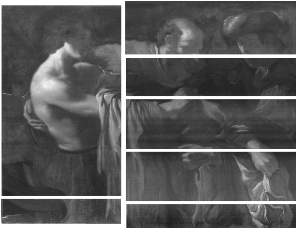
Fig. 4.11. Reflectographic images acquired by scanning device illuminating with lamps and no filters. Each image corresponds to one scan.
