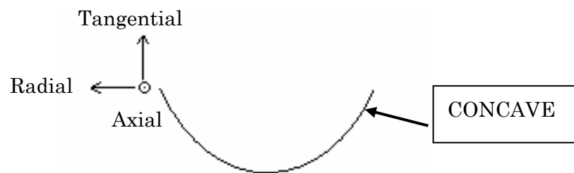
Fig. 4.6 – Test setup: triaxial concave accelerometers directions.
