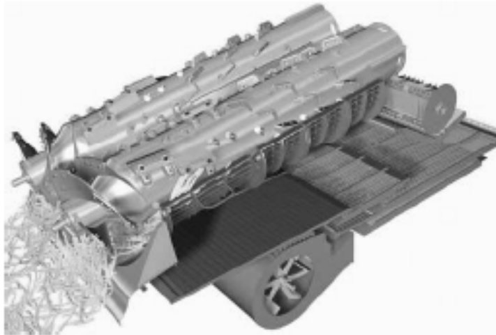
Fig. 1.3 – Longitudinal rotors in non-conventional combine harvesters.
