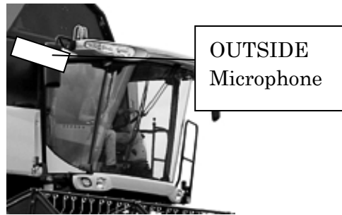
Fig. 4.5 – Test setup: microphone mounted OUTSIDE the machine, over the cabin.
