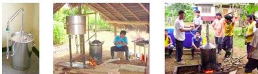
Fig. 29 Vapour hydro distillation apparatus: on the left, that used at “Centro de Acopio” Foundation Chankuap, Macas; and on the right that used at Wasakentsa reserve, Amazonian forest
