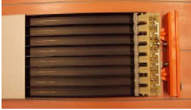
Figure 3.20: The mechanical structure of a BABAR LST.
