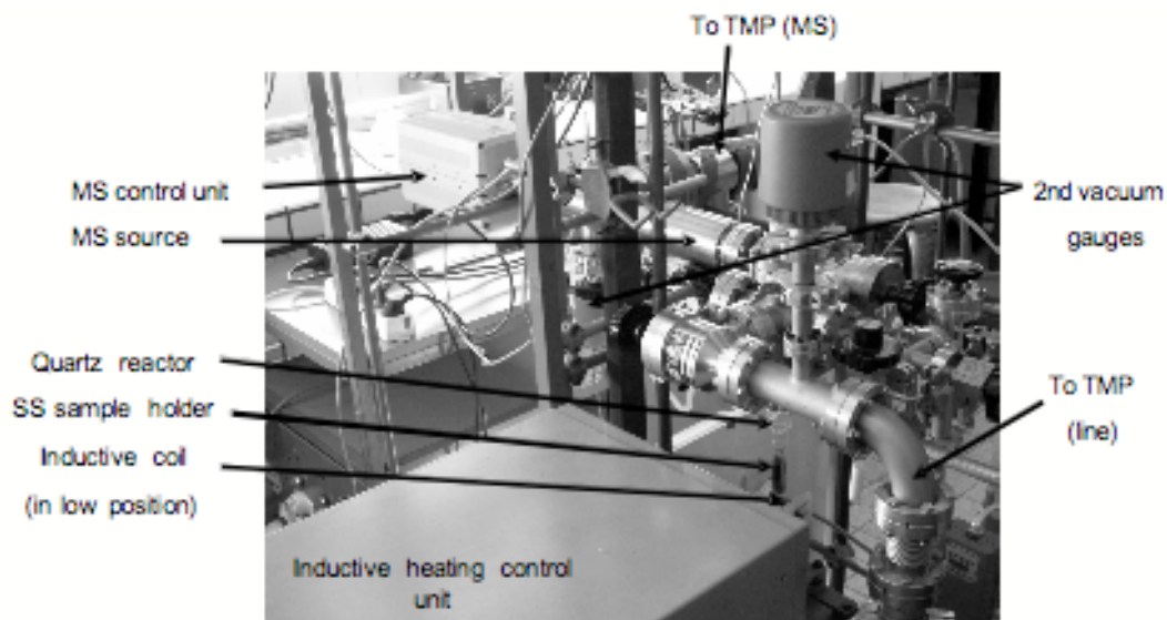
Figure 4.1: Picture of the experimental setup for vacuum TPD and ITPD.
