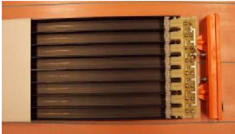
Figure 3.20: The mechanical structure of BABAR LST.
