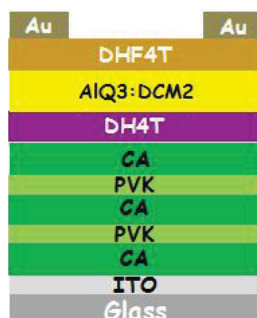
Figure 4.15: Structure of an OLET device with the gate dielectric composed of 5 layers of CA and PVK.
