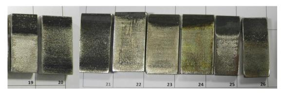
Figure 5.13: Samples after electropolishing, back from 19 to 26.
