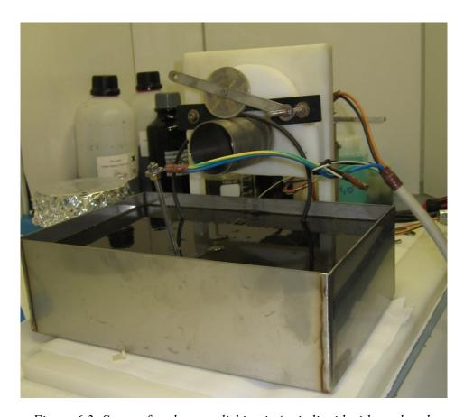
Figure 6.3: System for electropolishing in ionic liquid with steel tank.
