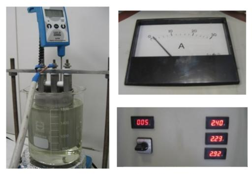
Figure 5.32: The electropolishing with rectifier.
