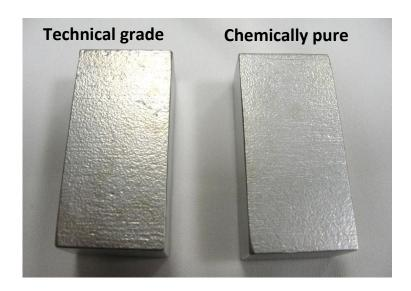
Figure 5.26: The samples after 90 minutes of treatment with the two different solutions.
