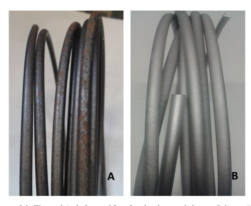
Figure 8.9: Wire rod A - before and B - after the electropolishing in Solution "S".
