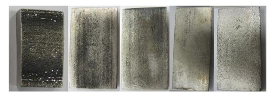
Figure 5.11: Samples after electropolishing, back from 41 to 46 (without 42).
