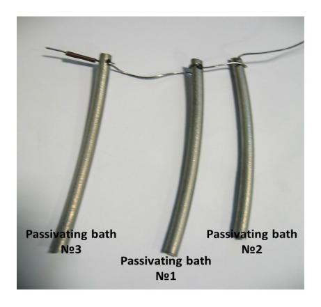
Figure 7.1: Samples passivated in different solutions.
