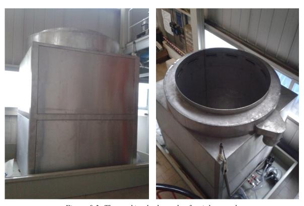
Figure 9.3: The working bath, made of stainless steel.
