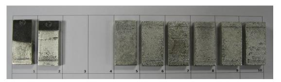
Figure 5.4: Samples after electropolishing, front from 1 to 10.
