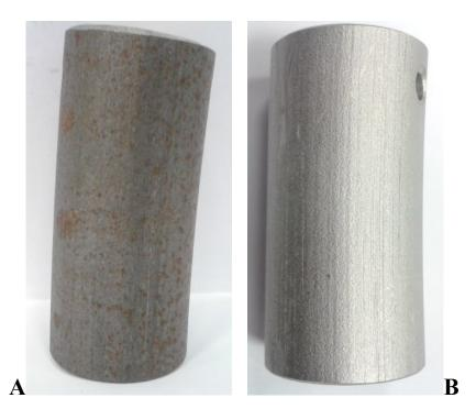
Figure 9.2: The stainless steel sample A- before and B- after electrochemical polishing
