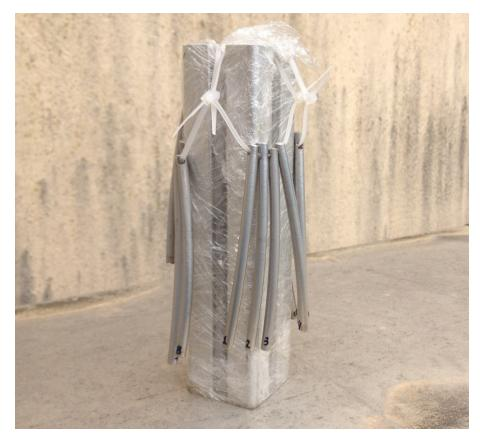
Figure 7.5: Samples passivated and left outside for 30 days.
