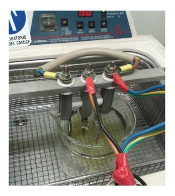
Figure 8.5: Electropolishing of stainless steel with ultrasound.
