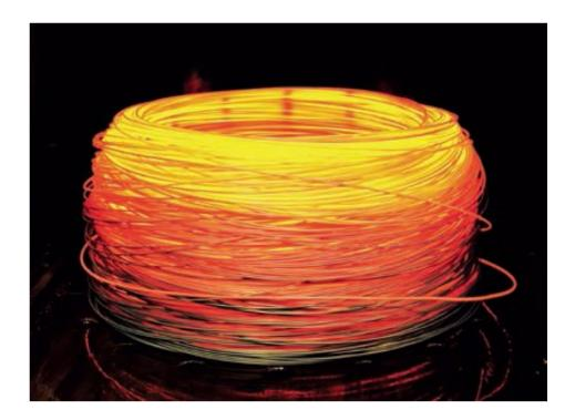
Figure 1.5: The hot rolled rod coil.
