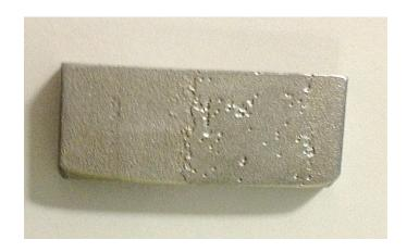
Figure 5.24: Sample of the martensitic steel after electropolishing.
