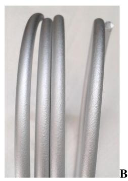
Figure 8.10: The steel coils after electropolishing in 100g/l Solution "S": A - at ambient temperature, B – at 70 °C.
