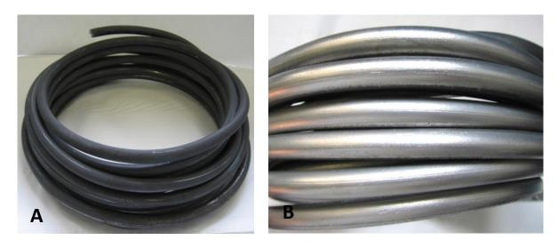
Figure 6.6: The rod with overlapped coils A- before and B- after electropolishing.
