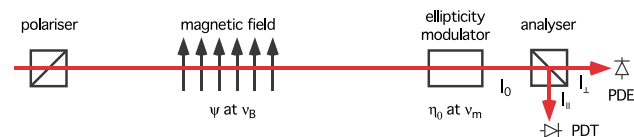
Fig. 1 A simple heterodyne ellipsometer. PDE extinction photodiode, PDT transmission photodiode
