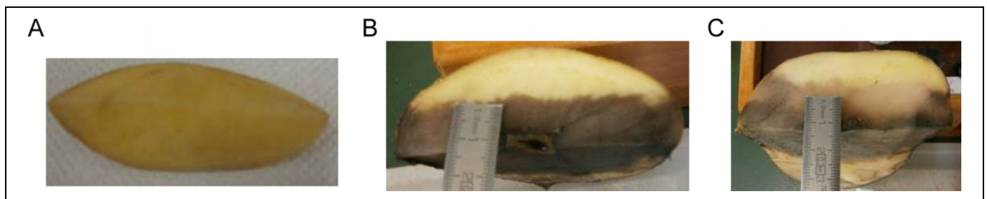
Figure 13. A, Potato tissue not electroporated after 24 hours. Effect of 10 V pulses on potatoes using the following 2 different electrodes: (B) electrode in Figure 1A supplied at 1000 V shows an electroporation depth of 1.2 cm and (C) electrode in Figure 1B supplied at 2000 V shows an electroporation depth of 1.8 cm.
