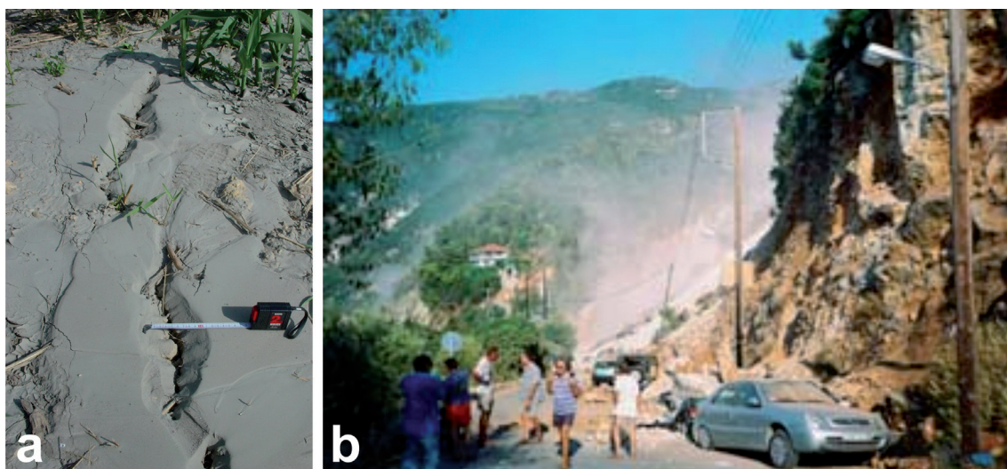
Fig. 3 - Examples of geological evidence used for the compilation of DaLO: a) ejected sand cones aligned along a ground fracture (June 8, 2008 Movri earthquake); b) earthquake induced rockfalls (August 14, 2003 Lefkada earthquake).
