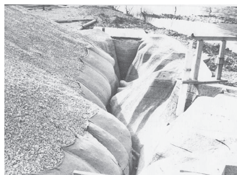
Fig. 15 - Original photo n.10, the landslide mass of gravel resting on the sliding surface, held in place by hemp nets and ropes, before a test of the second series (from GHETTI, 1962)
