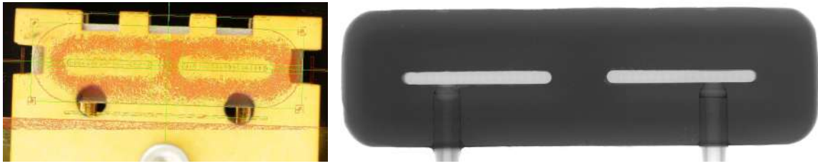
Figure 12. Left: image of a fluidic connector aligned in the horizontal plane with the corresponding solder layer on the silicon cooler, indicated with the red shadow. Right: X-ray of the solder joint attaching the fluidic connector to the microchannel cooler. No solder has entered the two inlet regions, and no large voids are seen in the solder layer.
