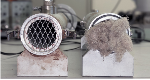
Figure 1. Loose hemp fibres and their installation in the plane wave impedance tube.
