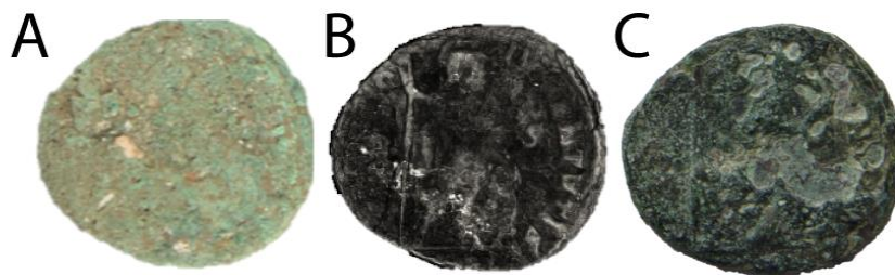
Figure 5 Reverse side of coin A3 (A) before cleaning, (B) virtually cleaned with \mu XCT and (C) after traditional cleaning. The loss of most of the figure of a soldier after the invasive cleaning is evident.
