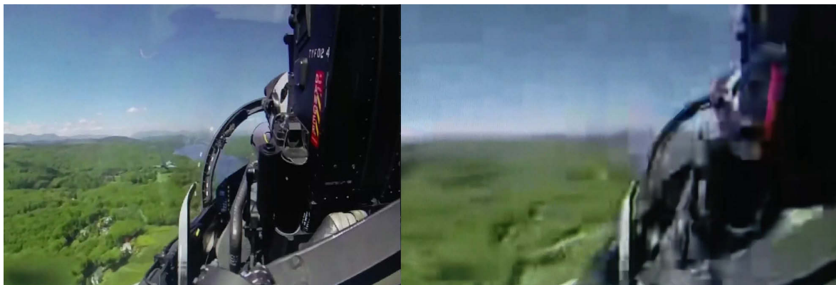
Figure 6.20: The left and right pictures show respectively a frame from a high and low video quality profile. As expected, pixelation is much more marked in the second frame.
