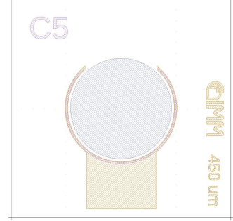
Mask 3: Diode active area
