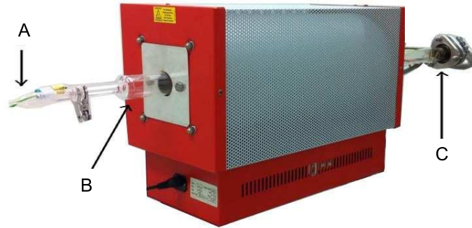
Figure 1.4: Hot wall furnace used for graphene synthesis. (A) indicates the port where gases are introduced, (B) is the quartz tube where the copper foil is placed, (C) is the furnace connection to the vacuum pump and way-out connection for exhaust gases.
