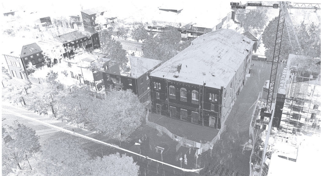
Fig. 5. View of the point cloud of the Novi Theatre. The data acquisition was carried out using Leica C10 and BLK360 laser scanners.
