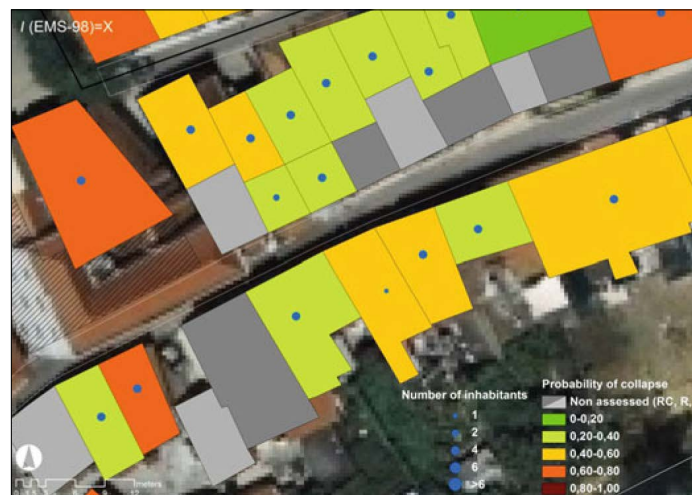
Fig.2. Seixal: mapping results for collapse probability and number of inhabitants for a Macro-intensity=X (Ferreira et al., 2013).
