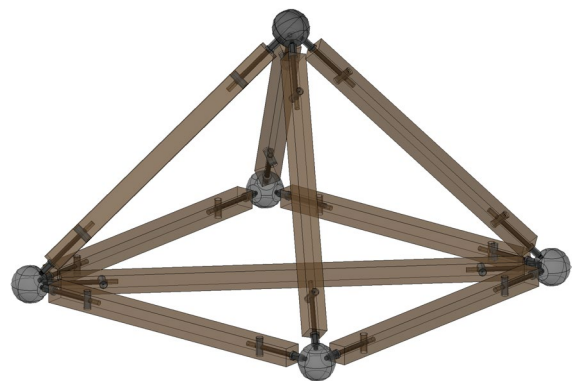
Fig. 3 Schematic representation of a timber structure with spheres and steel joints
