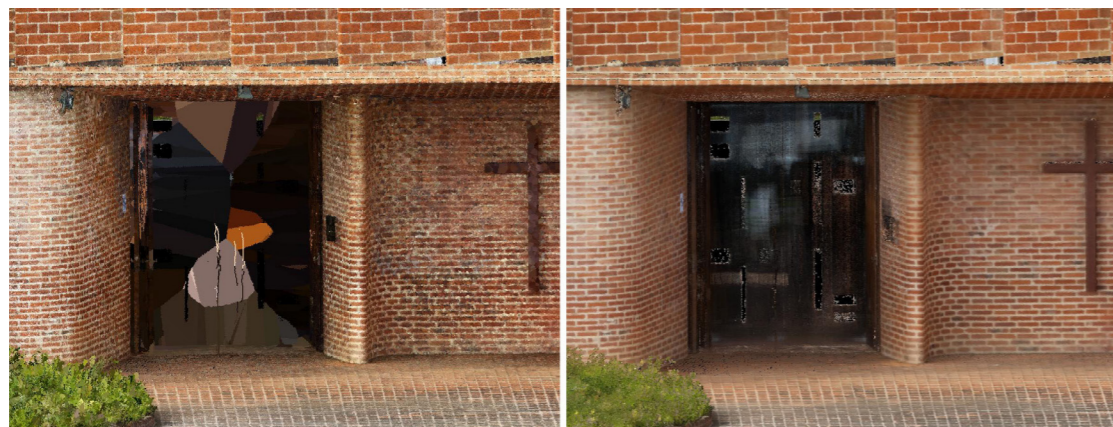
Fig. 6.04. Comparison of RGB data of laser scanner point cloud obtained through reprojection from photogrammetric point cloud (right) and from aligned images (left) in Christo Obrero Church in Atlantida dataset. With the first method some points were unreliable coloured, with the second the result improved.
