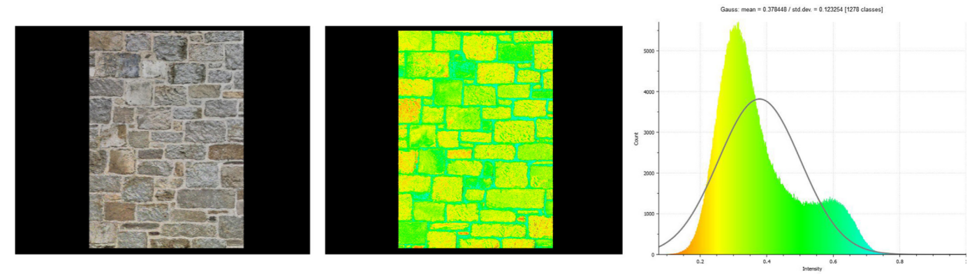
Fig. 6.12. St Margaret’s Church in Braemar. Comparative diagram for stone masonry. Histogram irregularities may be given by the different reflectance response between ashlar and mortar joints.
