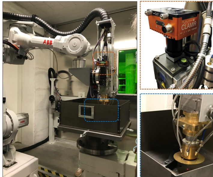
Figure 2.3 Robot used to fabricate the L-DED depositions with the CLAMIR camera illustration.
