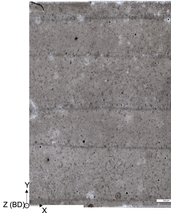
Figure 2.37 Micrograph of the top part of the multilayer specimen, also known as contour area.
