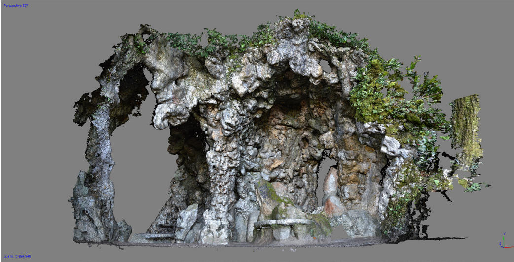
Fig. 3. Quinta da Regaleira in Sintra, The East Cave, point cloud obtained through a photogrammetric survey and processed through digital software. (Credit: Gennaro Pio Lento, 2019).
