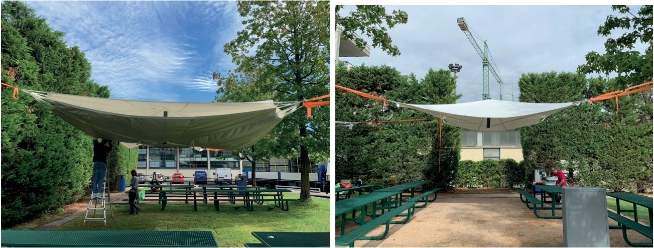
Figs. 21-22. Assembly of the temporary covers in order to measure the mitigation performances of the three kits on site, Politecnico di Milano Campus Bovisa, Milan – Italy, 2021 (Credits: ©Zanelli A.; Angelotti, A.; Viscuso, S.; Kutlu, A.).
