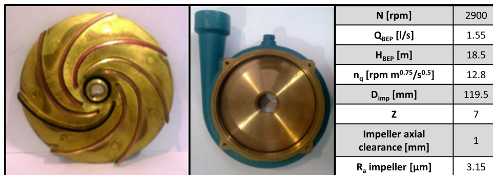
Figure 3. Centrifugal pump tested.
