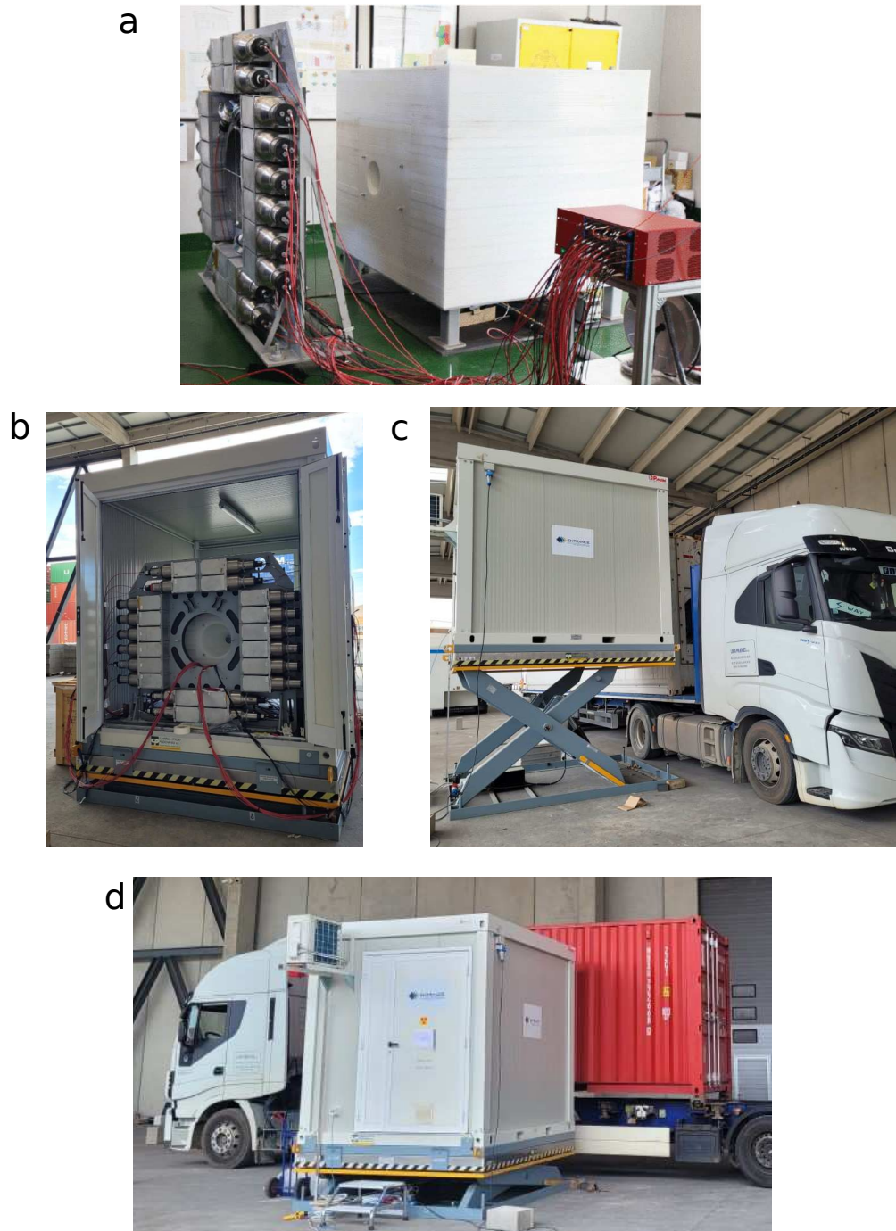
Figure 5.3: Configuration of the RRTNIS System: (a) RRTNIS at the Laboratory, (b)-(d) RRTNIS inside the external case and positioned on the lifter at different heights for container irradiation at the Rijeka Port
