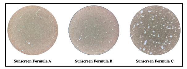
**Figure 1.** The coating based on Sodium Lauroy L Glutamate, Lysine that covers this type of commercial ZnO (Formula B) is able to optimize the wettability and dispersion of the powder in the chosen oily phase, as compared to uncoated ZnO (Formula A) or Zinc Oxide, Stearic Acid (Formula C).
