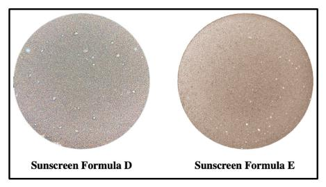
**Figure 2.** The data reflect the particle size of the two types of  $TiO_2$  used: in Sunscreen Formula D it is nanometric, while in Sunscreen Formula E the size of the aggregates (about 500 nm) is comparable with the wavelengths of visible light.
