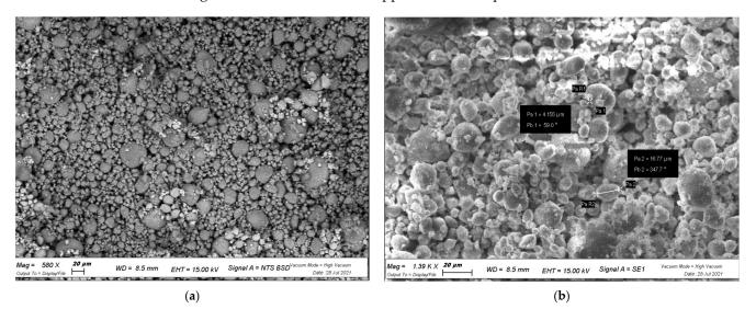
**Figure 6.** SEM image of non-nanometric Titanium Dioxide, Silica, Jojoba Esters at different magnifications: (a)  $500 \times$  magnification; (b)  $1390 \times$  magnification.
