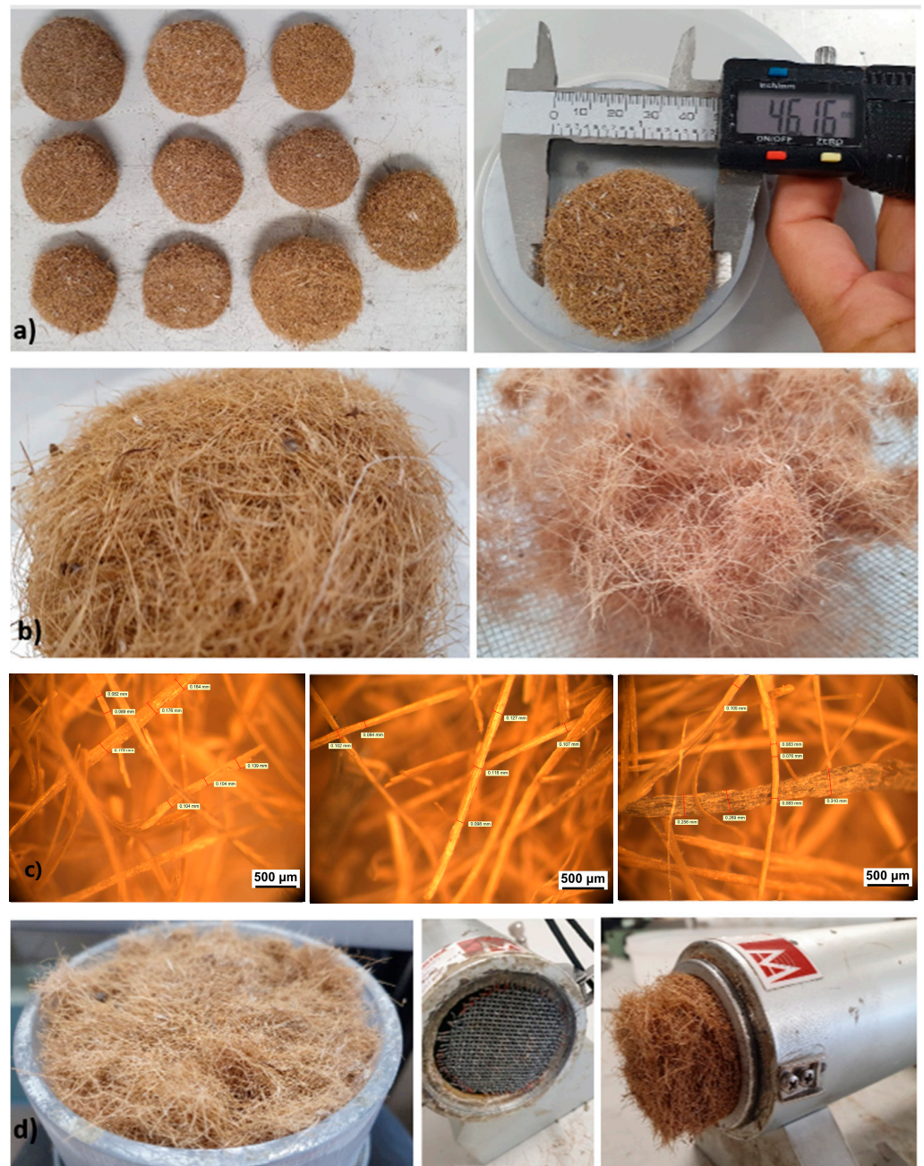
Figure 2. Collected Posidonia Balls (a), fibers obtained from the aggregates (b), microscope pictures of the fibers (c), fibers inside the sample holders for the measurement of airflow resistance (left) and sound absorption at normal incidence (right). In the center, the front grid for the compression of the sample (d).
