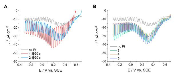
**Figure 5.** LSV of sensitized electrodes (**A**) NiO-B | **P1** | Pt-1 and NiO-B | **P1** | Pt-2 at 20 s deposition time and (**B**) NiO-B | **P1** | Pt-3–5 in N<sub>2</sub>-purged 0.1 M acetate buffer at pH 4 under chopped irradiation (in every graph, a comparison is made with the blank non-platinized electrode, grey trace).
