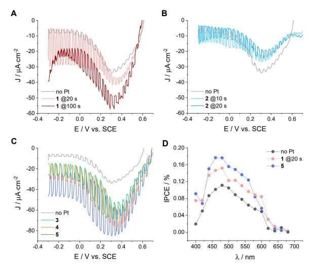
**Figure 4.** LSV of sensitized electrodes: (**A**) NiO-A | **P1** | Pt-**1**, (**B**) NiO-A | **P1** | Pt-**2**, and (**C**) NiO-A | **P1** | Pt-**3**–**5** in N<sub>2</sub>-purged 0.1 M acetate buffer at pH 4 under chopped irradiation (in every graph, a comparison is made with the blank non-platinized electrode, grey trace); (**D**) photoaction spectra of NiO-A | **P1** | Pt-**1** at 20 s deposition time, NiO-A | **P1** | Pt-**5**, and the blank non-platinized electrode.
