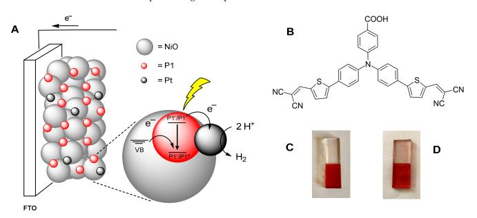
**Figure 1.** (**A**) Pictorial representation of the NiO photocathode and the related mechanistic pathways towards hydrogen evolution; (**B**) molecular structure of the **P1** dye; pictures of a sensitized NiO electrode of (**C**) type A and (**D**) type B.
