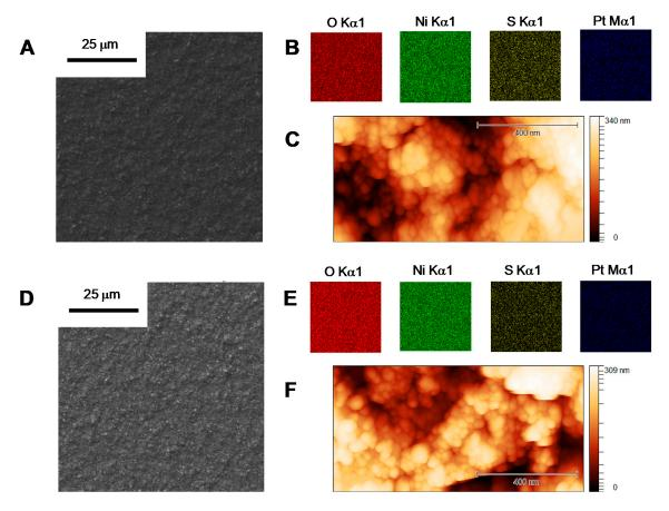
**Figure 3.** SEM micrographs (**A**,**D**), corresponding EDS elemental maps (**B**,**E**), and AFM images (**C**,**F**) of sensitized NiO electrodes of type A after Pt deposition using Method 1 at 20 s deposition time (**A**–**C**) and Method 5 (**D**–**F**).
