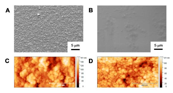
**Figure 2.** SEM micrographs (**A**,**B**) and AFM images (**C**,**D**) of NiO electrodes of type A (**A**,**C**) and type B (**B**,**D**).
