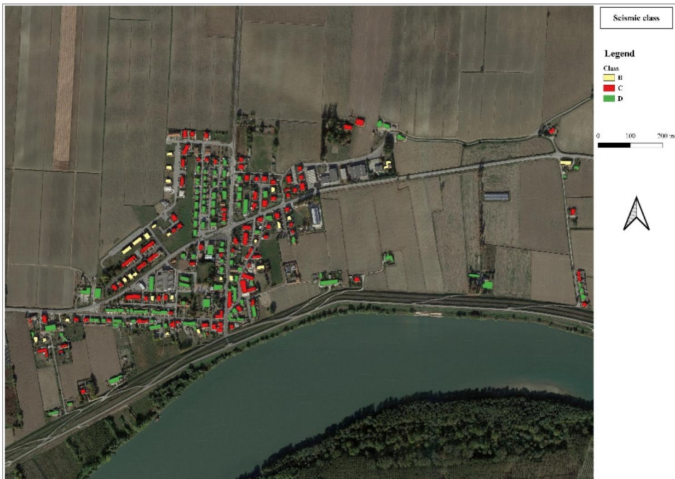
Figure 10. 1:5000 scale map showing the cataloging of buildings according to seismic risk class.
