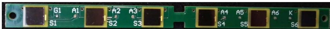
Figure 5.2: Picture of the front of one PCB used in the CACTUS apparatus. The G1 pin is the common ground, the K pin is the common anode and the pins A1-A6 are the six anodes of the sensors. The labels S1-S6 mark the six sensors in ascending order.
