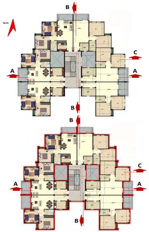
Figure 1 Case study floor plan before (above) and after adding insulation around external walls (below)
