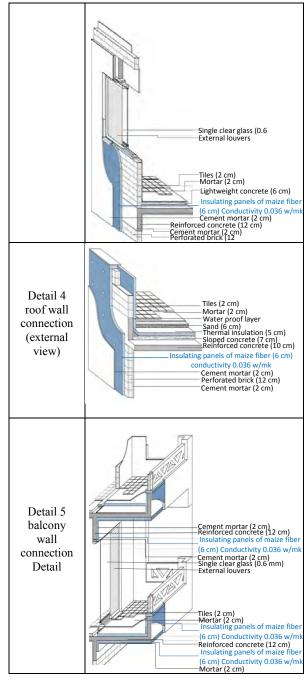
Table 6 External wall layer properties after adding insulation of maize fiber
