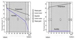
Figure 3 Thermal behaviour of the external wall during the lowest recorded temperature (on the left) and the highest recorded temperature (on the right)
